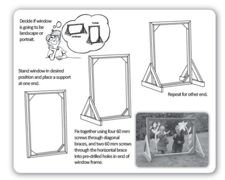
Minimum of 2 people required. Check all parts are present. Read through the instructions before you start. Lay panels out close to where assembled unit will be positioned.
